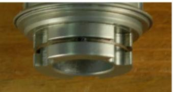
Step 5: To reassemble the pawls make sure the spring indents with the tiny pin that is in the spring groove. This is critical or the pawls won't work.
