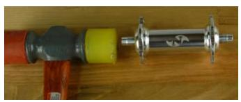
Step 3: Knock the other bearing out the same way. This will complete disassembly of the hub.
