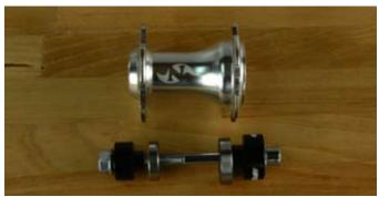
Step 17: The photo at left shows the correct stack for the press on step 18. It should be obvious which press to use with each bearing as they are different sizes. The OD of the press should match the OD of the bearing.
