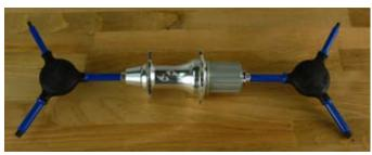
Step 1: To disassemble the rear hub put two 5 mm allen keys in the two threaded axle end caps and unscrew. Don't stick the allen keys in too far or they can go into the end of the broached axle. If they don't unscrew pretty easily this is probably what is happening.
