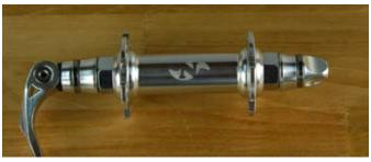
Step 4: To assemble it, slide the bearings over the end of the axle while the axle is in the hub. Using two nuts or other spacers (which come with the bearing press) squeeze the bearings in with the quick release lever. If the axle is too tight knock it a bit with the rubber mallet. If it's too loose squeeze it some more with the skewer.
