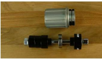
Step 13: To replace the bearings, use the bearing drifts to put the bearing back in. The photo at left show the way the drifts are stacked to complete step 14. It is imperative that the drift that holds the bearing on the inner diameter is used to slide the bearing in.
