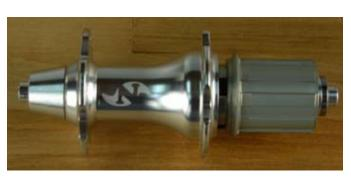
Step 20: Slide the axle assembly through the hub and thread on the non drive side end cap until you take up all of the play. The cassette body may slide right into the drive ring or it may not. If it doesn't, rotate the cassette body counter clockwise as you push the pawls down with a small screw driver. That should index them so the cassette body slide in. Tighten the two end caps very snug with 5 mm allen keys.
