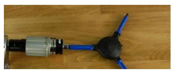
Step 16: Press the bearings in only until they are just barely snug. Too tight and the sleeve won't slide and it will be hard to slide in the axle. Too loose and it will cause the hub and cassette body to be out of adjustment. This is the only hub adjustment that requires any type of feel. You won't know if it's right until the hub is assembled.
