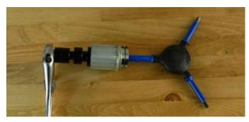
Step 12: Use the bearing drift to pull the inboard bearing out of the cassette body
