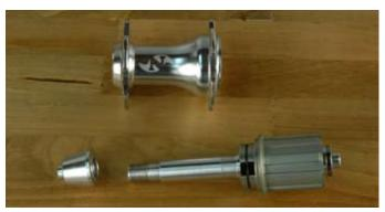
Step 18: Slide the cassette body onto the axle and install the threaded drive side axle end cap finger tight. Oil the pawls (or use a very light grease)
