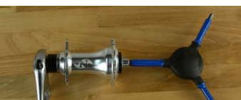
Step 17: Press the bearings in until snug. No need to overtighten.
