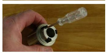
Step 4: Remove the pawls by putting a small flat bladed screw driver under one pawl and pry it up. This will loosen the pawls and springs. Clean them off making sure there is no degreaser left on them before reassembly.
