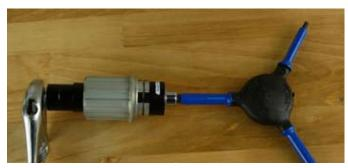
Step 14: Press the bearing in until snug. You are going through two press fits here. There is no need for a lot of pressure on the bearing after it seats.
