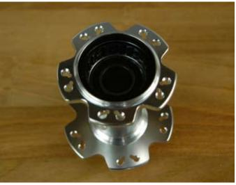
Step 19: Use a thick grease in the drive ring pictured at left. NOTE: Don't use a grease that will freeze in the winter if you ride in cold climates. I use the Morningstar grease for maintenance. It's really expensive but it's the best.
