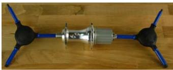
Step 2: After you have removed one end cap, unscrew the other one. The ends of the axle are broached to accept a 5 mm allen key.
