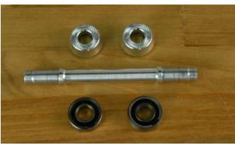
The parts at left are all the parts for the front hub. There are two end caps, the axle and two R6 bearings. If you need these please send me an e-mail pricing is on the spare parts page linked on the wheel pages.
