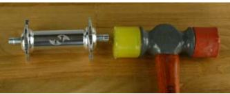
Step 2: Knock the axle out using a rubber mallet. If you don't have one a block of wood will also do the job.
