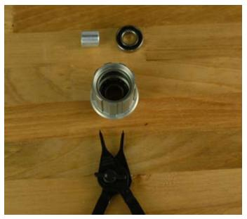
Step 11: Step 10 will dislodge the bearing and the spacer. You will need need to use a snap ring plier to remove the snap ring holding the other bearing in the cassette body.
