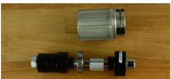
Step 15: The photo at left shows the stack to press fit the bearing in step 16. Note the sleeve in the center.
