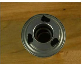
Step 9: To remove the cartridge bearins from the cassette body, look in the cassette body and notice the sleeve that is in between the two bearings. Push it over to one side so you can access the outboard bearing with a drift punch.
