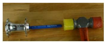
Step 7: To remove the hub cartridge bearings, knock the drive side bearing out with a drift punch trying to make sure you hit the innder race of the bearing.
