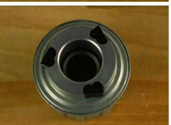
Step 6: Slide the pawls under the spring by holding the spring up with the same small flat bladed screw driver. The pawls should spring up like the photo at left.
