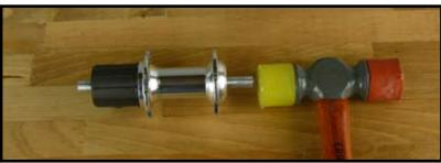
**Step Four** Using a rubber mallet or block of wood, drive the cassette body cartridge bearin out of the drive side by hammering on the axle.
