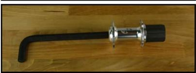
Step Five DO THIS ONLY IF YOU WANT TO REPLACE THE CASSETTE BODY. Using a 12 mm allen key unscrew the cassette body nut. Note you will need to do this with a completely built wheel. Trying to do it with the hub only as pictured at left is impossible because the nut is on there too tight. To replace the cassette body tighten with the same 12 mm nut and wrench.
