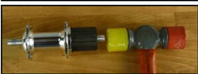
**Step Two** Using a rubber mallet or a block of wood, hammer out the non drive side cartridge bearing.
