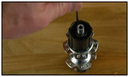
**Step Eight** Push the rubber seal into the cassette body with a small flat bladed screw driver until it is seated against the bearing. If it's not in far enough it can come into contact with the cassette lock ring.
