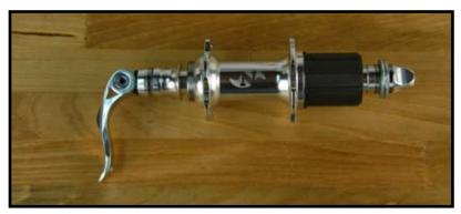
**Step Seven:** Using 3/8" washers that fit over the axle and inside the bearing seats, put both cartridge bearings in their bearing seats slide on the washers and the axle end caps and use the quick release to press in the bearings. The washers come with the Neuvation replacement bearing kit.
