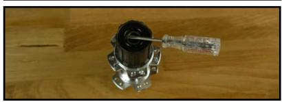
**Step three** Using a small bladed screw driver pop out the drive side rubber seal.
