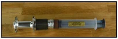
**Step Six:** Normally all you want to do is relube the cassette body. To do this you need a Morningstart freehub buddy. That is pictured at left with the Morningstar grease. Squirt grease in until it comes out near the hub shell.
